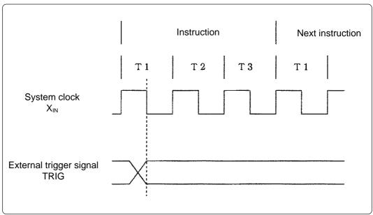
Figure 6.2 Latch timing of the external trigger signal
